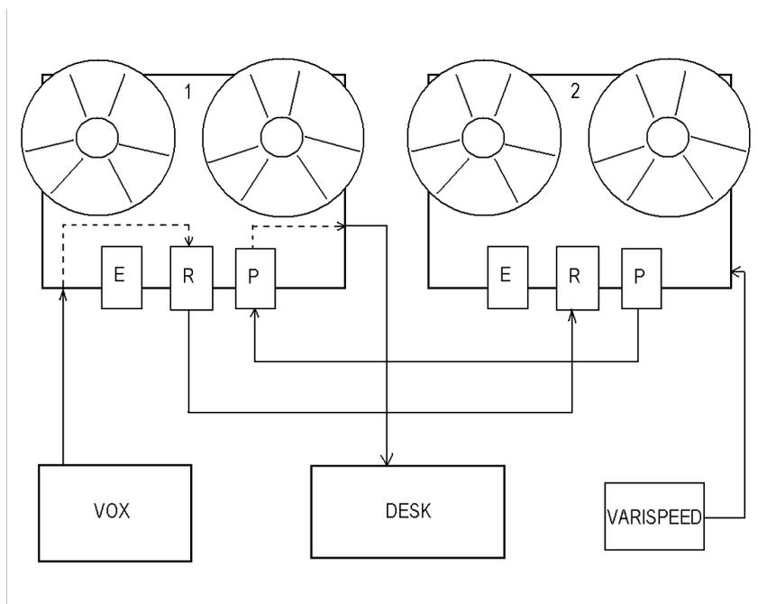
Figure2: Two tape decks connected in order to get the ADT. The playback head of deck 2 is connected to the record head of deck 1.
